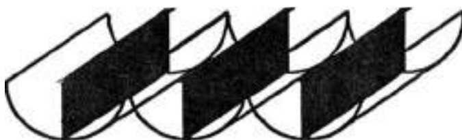
Figure 4.6 A highly efficient solar power system comprising bifacial solar modules and hemispherical compact mirrors, resulting in more electrical power output per module, with large space saving.
